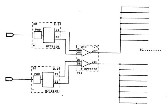
EACH BUFFER DRIVES UP TO AND INCLUDING 9 LOADS - THIS 15 LOAD OUTPUT IS SPLIT BETHEEN TWO BUFFERS
