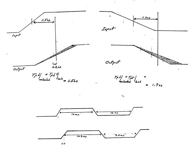
Effect of loading on the rise and fall edges for a single macro, 4 loads. Unloaded Tpd = 1.3ns. Loaded, Tpd (+) = 1.5ns; Tpd(-) = 1.7ns. Pulse shrink is at signal = low at 9.8ns; pulse stretch is at signal = high at 10.2ns.
