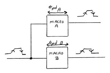
$\Delta t_{p}J + \equiv \Delta t_{p}J - \left| t_{p}J_{A} - t_{p}J_{B} \right| = 0.2 * t_{p}J_{A}$ (Acr B)
