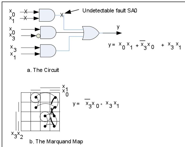
Figure 12-1 Redundant Circuit
