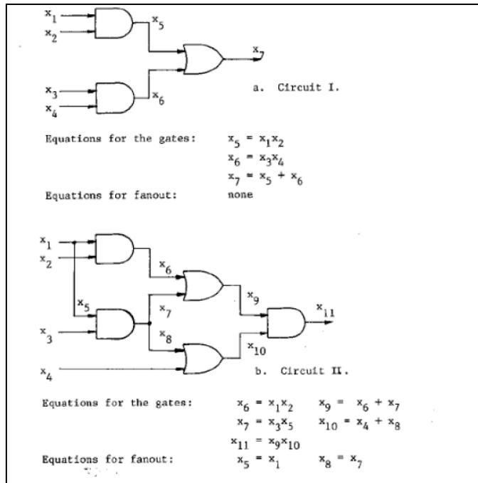
**Figure 12-3 Examples of Labeling; Equations**
