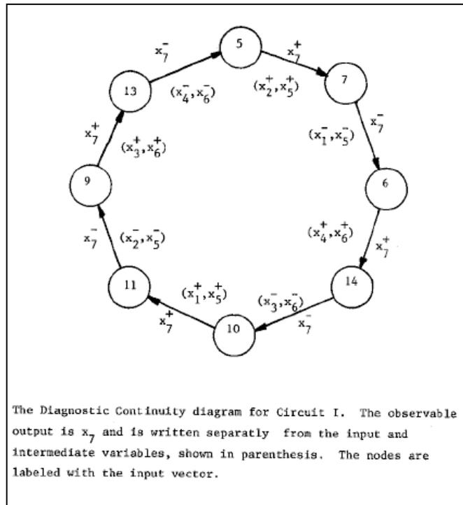
**Figure 12-7 Diagnostic Continuity Diagram**
