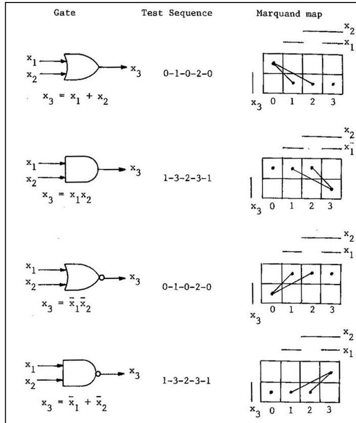
Figure 12-8 Test Sequences for Elementary Gates
