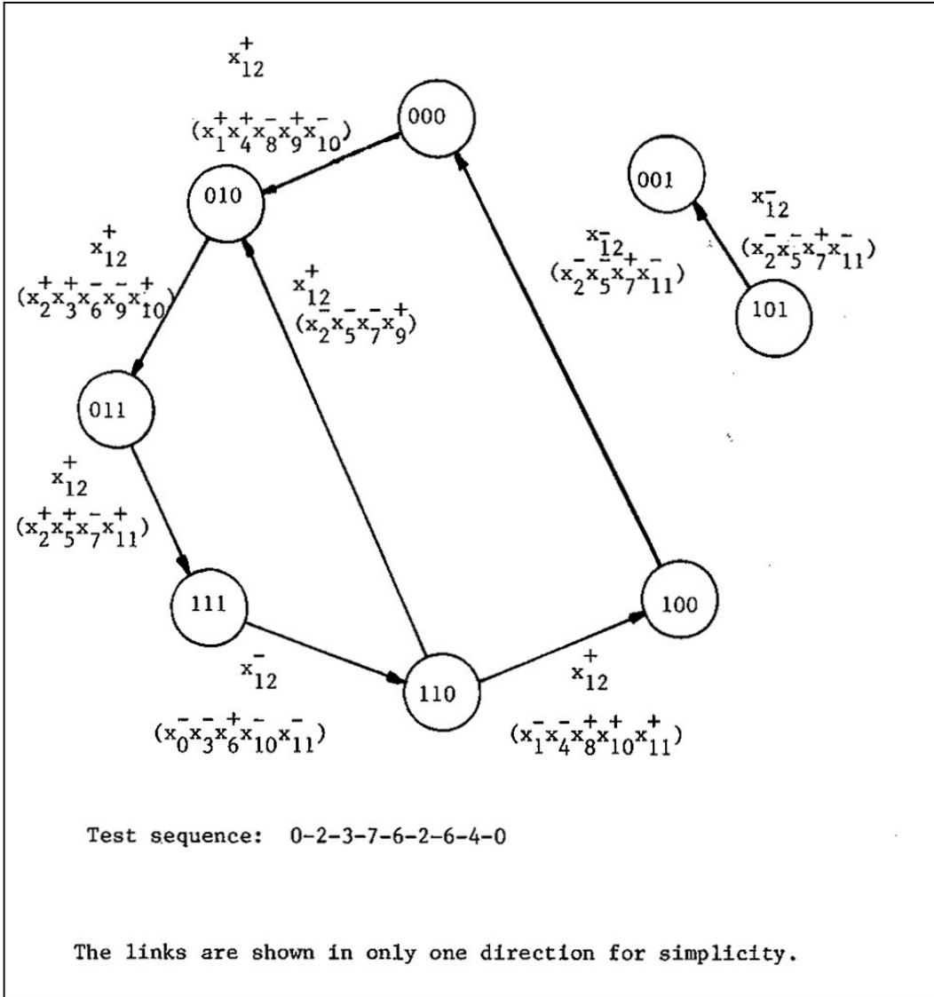
Figure 12-17 Diagnostic Continuity Diagram for Figure 12-16
