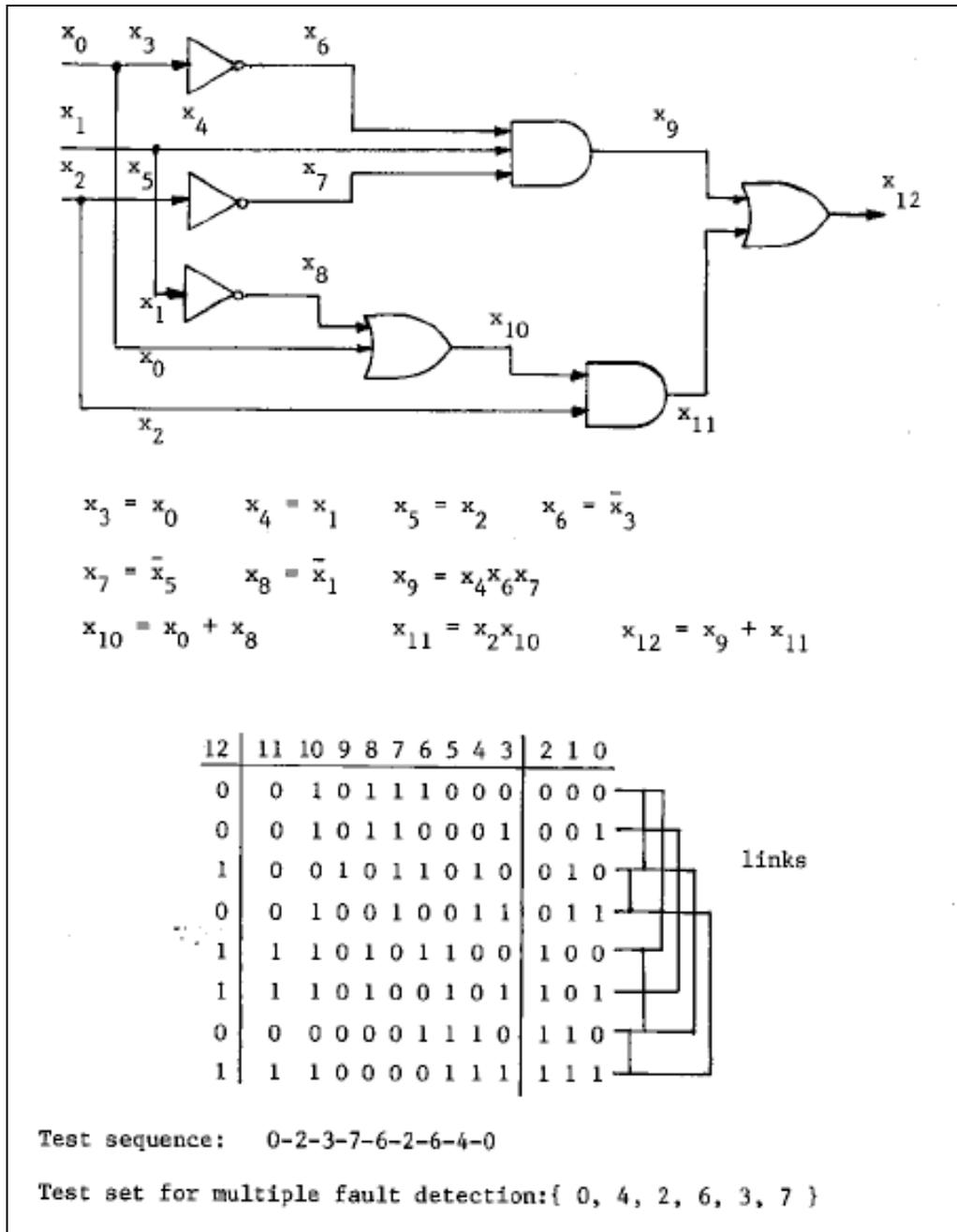
Figure 12-16 Multiple Fault Testing Example from Yau and Tang (see references)
