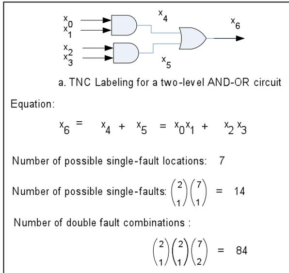
**Figure 12-2 Sample Circuit used in Comparing Methods**
