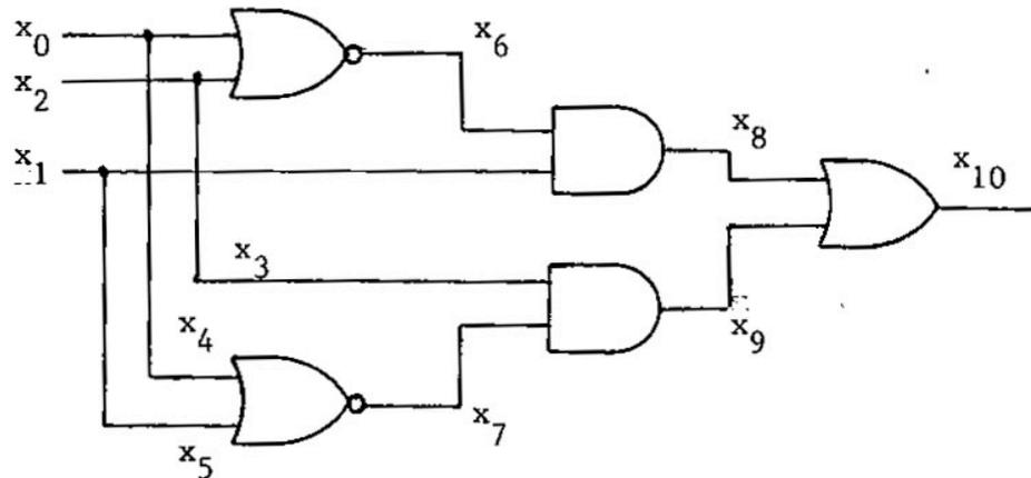
$$x_{10} = f = \bar{x}_2 x_1 \bar{x}_0 + x_2 \bar{x}_1 \bar{x}_0$$
